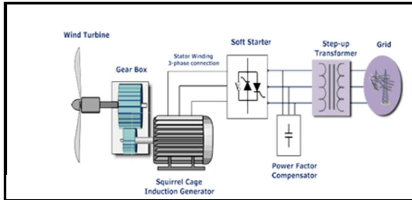
Figure. 4 Fixed speed control SCIG based connected WECS
