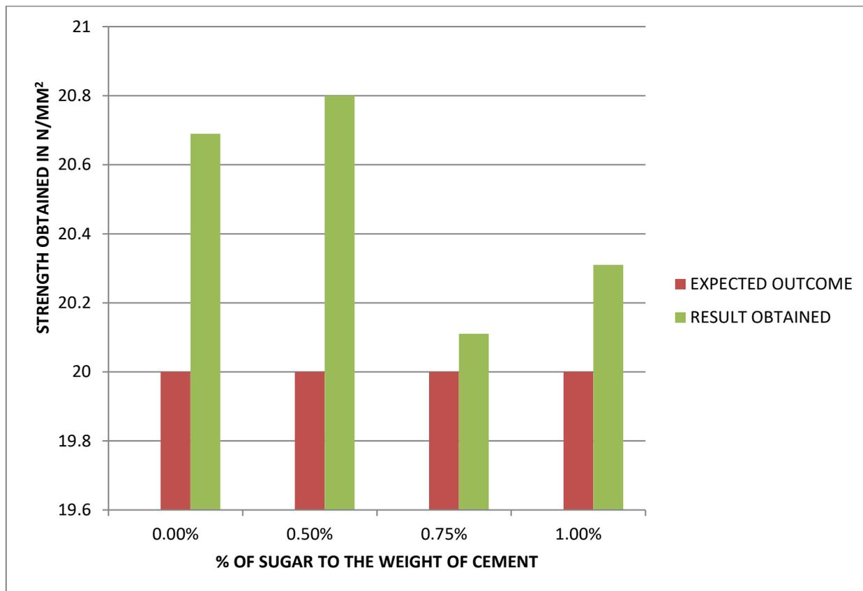
**Figure 8.** Compressive Strength and Percentage of Sugar Content
