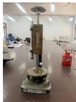
**Figure 2.** Vicat's Apparatus
